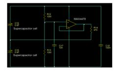
Figure 5: Low-current active-balance circuit
