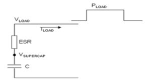
Figure 7a : Model for solving the constant power case Circuit.
