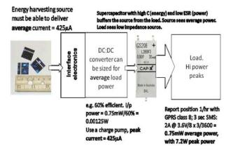
Figure 3: Supercapacitor as a power buffer
